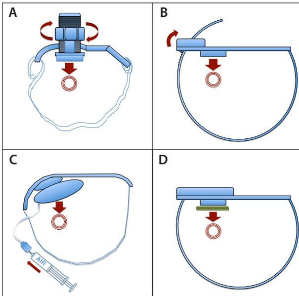
**Figure 1.** Different designs and technologies for compression wristbands: mechanical compression through a screw press (A), mechanical compression through a band-tightening press (B), pneumatic compression through an inflatable air bladder (C), and additional implementation of a hemostatic pad for faster hemostasis (D).
